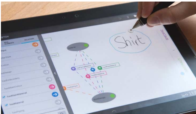
Figure 9: OntoSketch implemented on an Android based tablet-PC enabling pen and multi-touch interaction.
